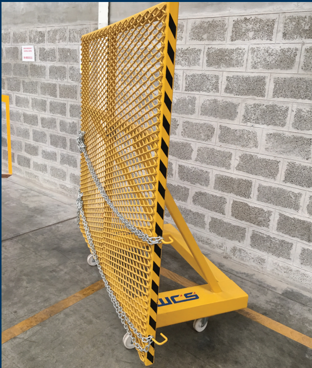
A chain enables the screen to be fixed to the machine for maximum protection. Wheels allow for greater mobility.
